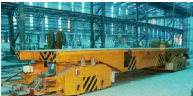
130MT Flat Bed Transfer Car with Underground Bus Bar
