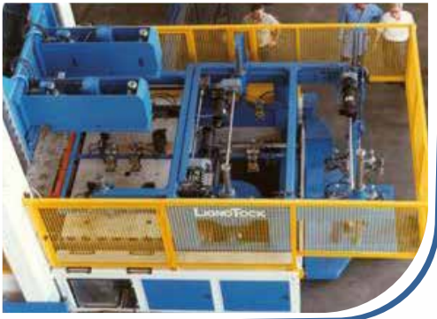
Automated blank feeder with steaming unit and pre-forming brackets.
