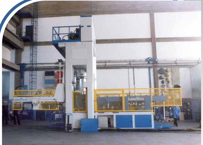
LIGNOTOCK automated motor vehicle door panel production line. C.R.ligno.6,000 kN press. Forty systems delivered in Germany, the U.K., Spain and the United States.
