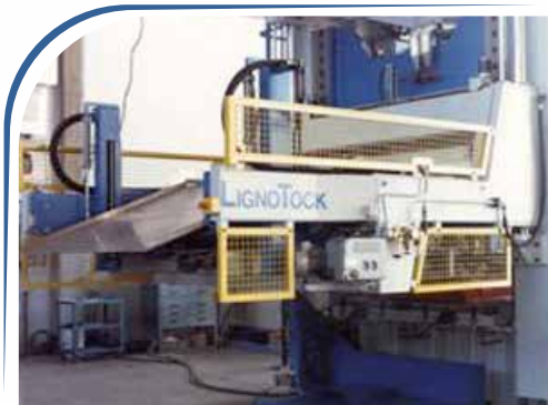
Automated clip feeder and finished part unloading.
